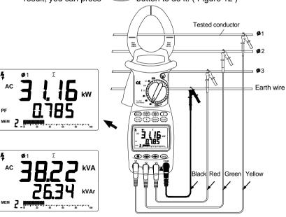
(Figure 12.The First Phase Power Measurements)
