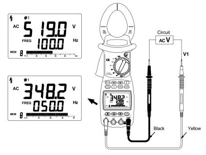
(Figure 3. Voltage Measurements)
