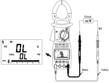
( Figure 4. Voltage Exceeds 600V )
