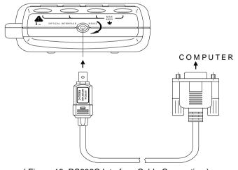
(Figure 18. RS232C Interface Cable Connection)
