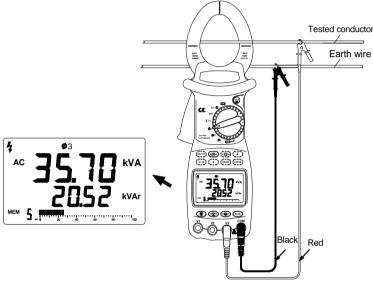
(Figure 10.Apparent power measurements)
