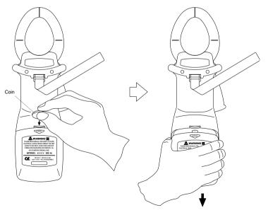
(Figure 23. Open The Battery Cover)
