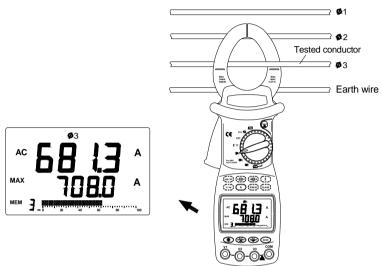
(Figure 6. Maximum Value Of Current Measurements)
