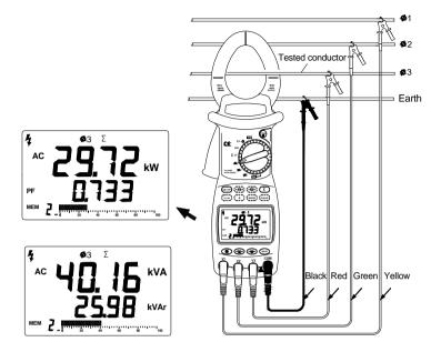
(Figure 14. The Third Phase Power Measurements)
