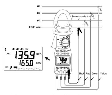
(Figure 16. Total Apparent Power Of Three-Phase)
