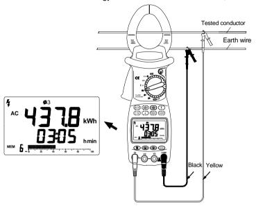
(Figure 11. Active Energy measurements)
