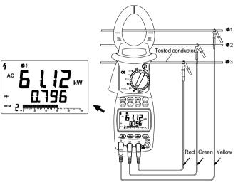
(Figure 17.Power Measurements Of Three-Phase Three-Wire)
