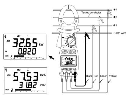
(Figure 13.The Second Power Measurements)
