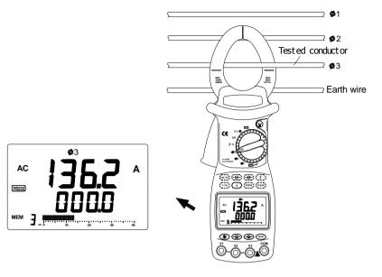
(Figure 5. Current Measurements)
