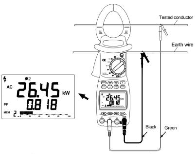
(Figure 8. Single-phase Power Measurements)
