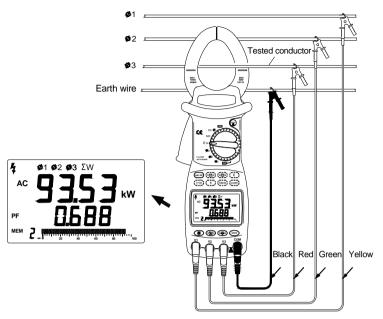
(Figure 15. Total Active Power Of Three-Phase)
